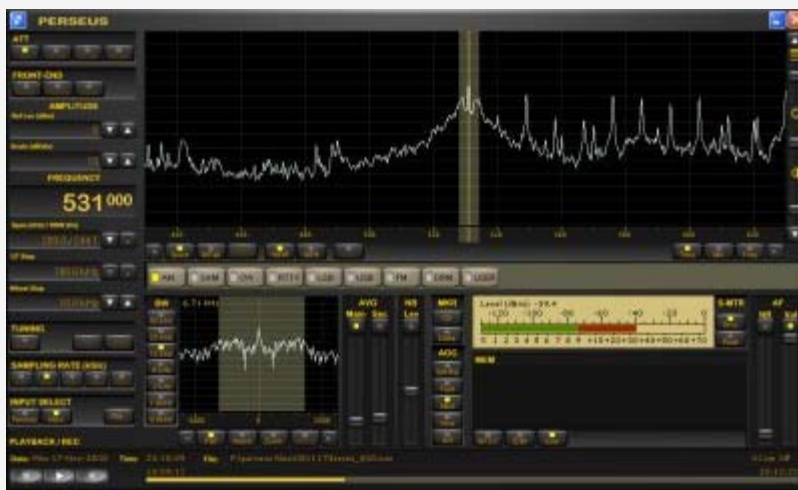
Waterfall View during excessive splatter, and after adjustments using Perseus SDR software. Click to enlarge. Sorry screen is smaller than the image. This is to accommodate 800 by 600 screens
