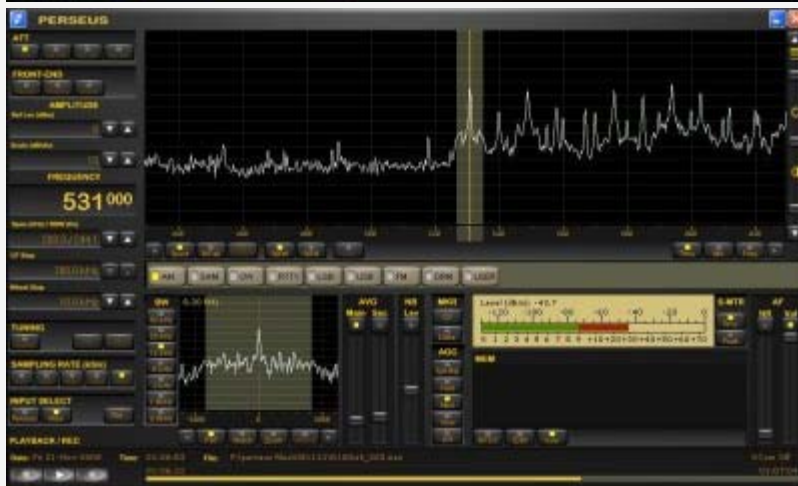
Spect View during excessive splatter, and after adjustments using Perseus SDR software. Click to enlarge. Sorry screen is smaller than the image. This is to accommodate 800 by 600 screens
