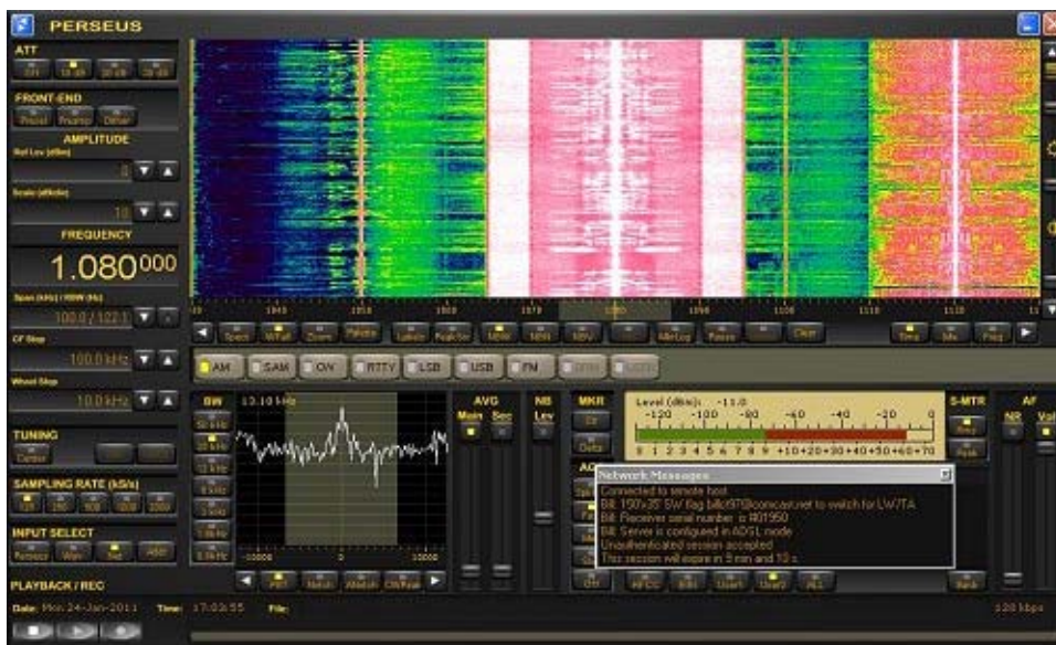
An example of a Perseus Server in CT, USA. Note the IBOC on WTIC 1080
