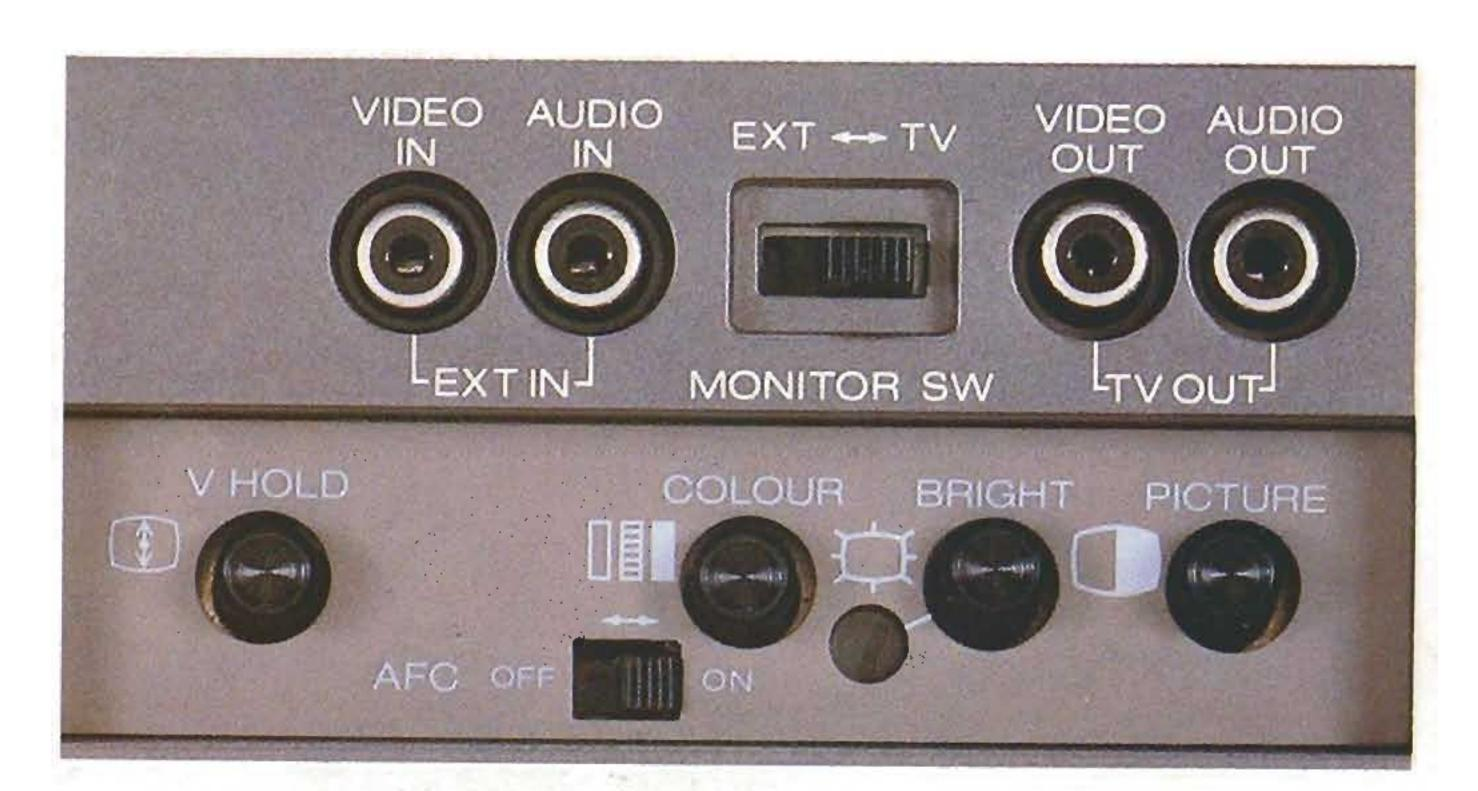
Video external input: 1 Vp-p 75 ohms Video TV output
