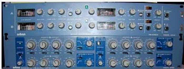
The ORBAN notch filter is the bottom unit
